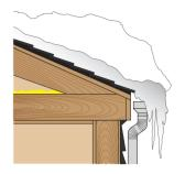
When snow and ice melt, trapped water can infiltrate to damage the roof deck and building interior.
